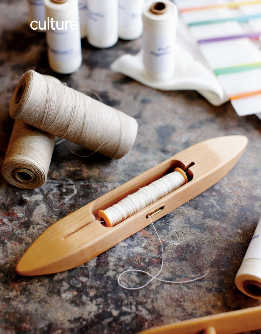
In order to create the woven part, or weft, the wooden shuttle is fed through vertical threads called the warp. Laskey colors her threads by dipping them in a dye bath and names the final piece after the manufacturer's paint color. ABOVE At work at her 1970s loom. BELOW An assortment from Laskey's shuttle collection.
