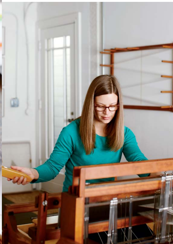
In order to create the woven part, or weft, the wooden shuttle is fed through vertical threads called the warp. Laskey colors her threads by dipping them in a dye bath and names the final piece after the manufacturer's paint color. ABOVE At work at her 1970s loom. BELOW An assortment from Laskey's shuttle collection.
